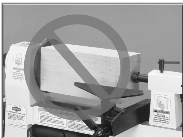
Figure 17. DO NOT attempt to turn workpieces thicker than 2" x 2" without first cutting the corners off!
